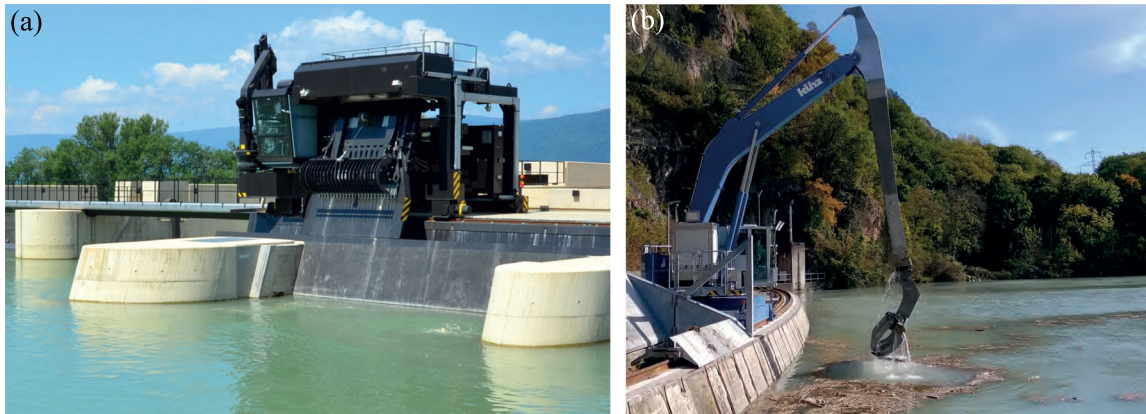
Figure 8.6 (a) Cable operated rack cleaning machine, (b) hydraulic cleaning machine with a flexible, tilting arm (photos by kuenz GmbH)
