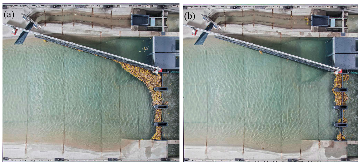
Figure 2.16 LW accumulations at the louver with \alpha = 30^\circ in the physical model (1:35) of a Swiss run-of-river HPP after the simulation of a 100-year flood event if (a) turbines are in operation and (b) turbines are shut down during the flood event; adapted from Kriewitz (2015)
