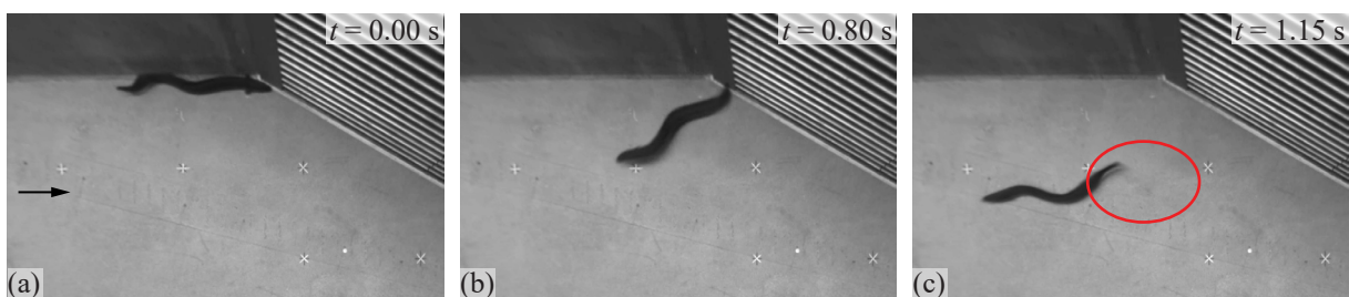
Fig. 8.11: An eel with TL = 61 cm which approached the HBR with negative rheotaxis and escaped upstream, while it lost a dark fluid (encircled in red) after it was exposed to rather large voltage gradients at the upstream rack end (Video: http://dx.doi.org/10.3929/ethz-b-000450740 )
