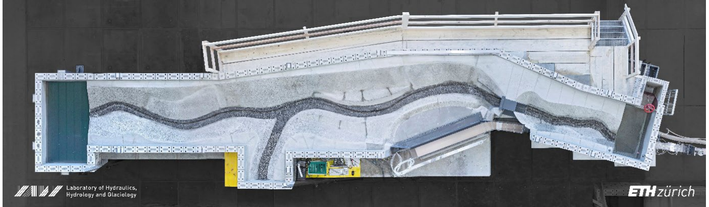
Figure 1: Physical model of the inlet area at a scale of 1:20
