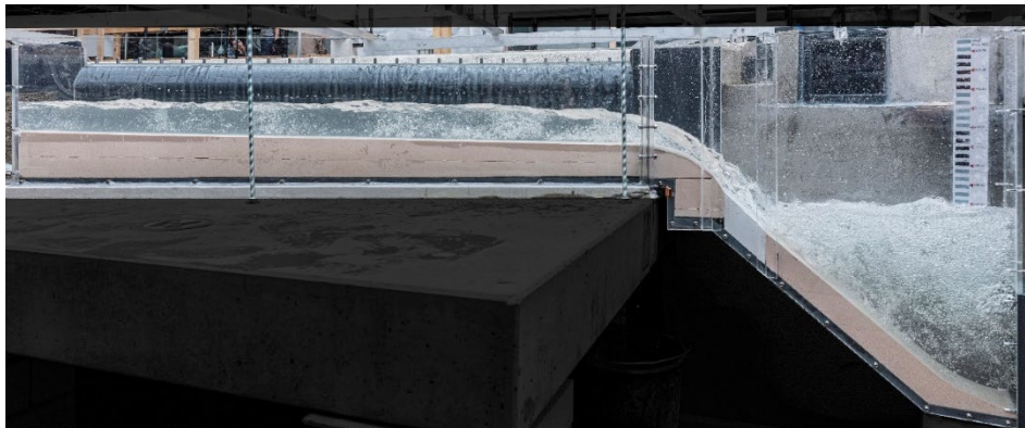
Figure 2: Side channel and drop shaft of the diversion tunnel with high air entrainment at HQ 100
