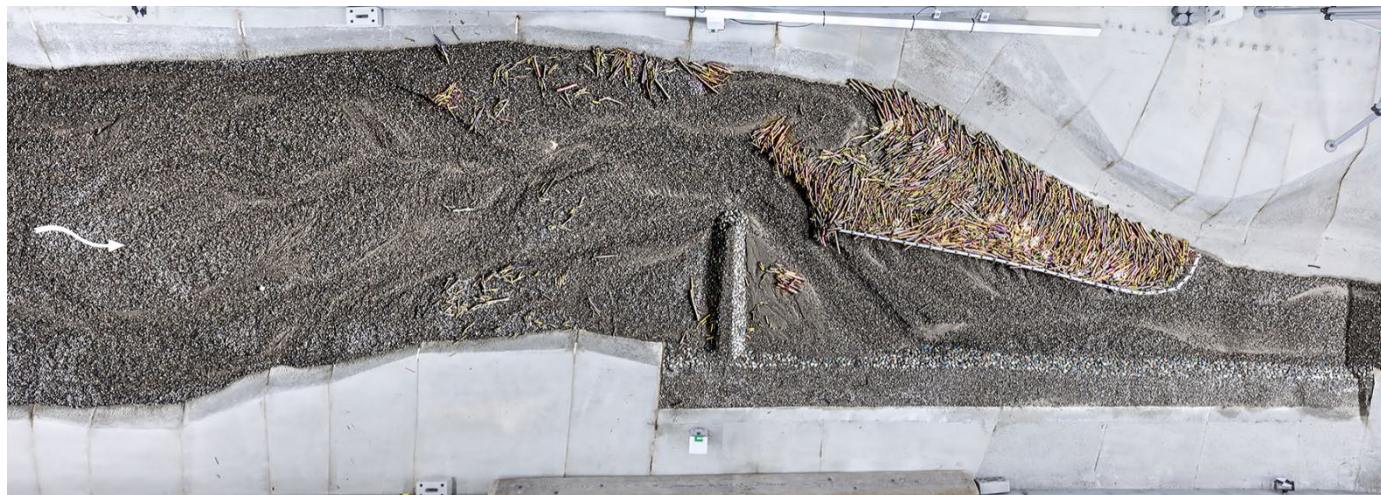
Depositions of large wood in the retention rack after the design event (100-year flood).
