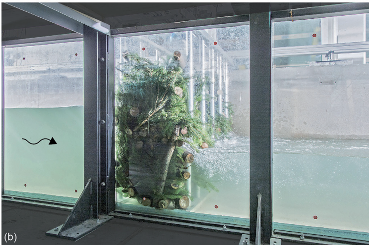
Close-to-prototype-scale experiments on resulting backwater rise \Delta h (a) without and (b) with 15% organic fine material
