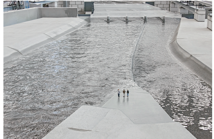
Fig. 2: View of the representation of Zurich main station in acrylic glass, seen from the confluence with 'Schanzengraben'
