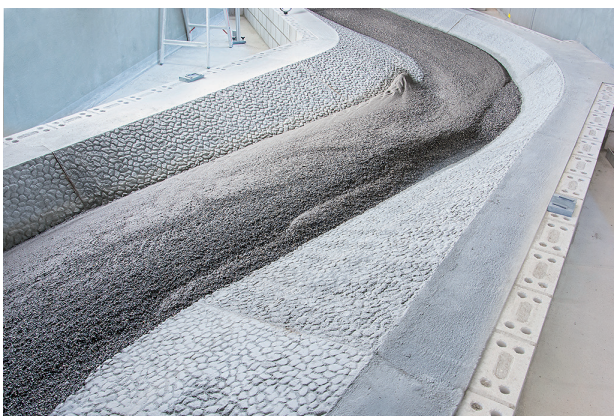
River bed with point bar and scour in the second bend (Picture: A. Schlumpf, VAW)
