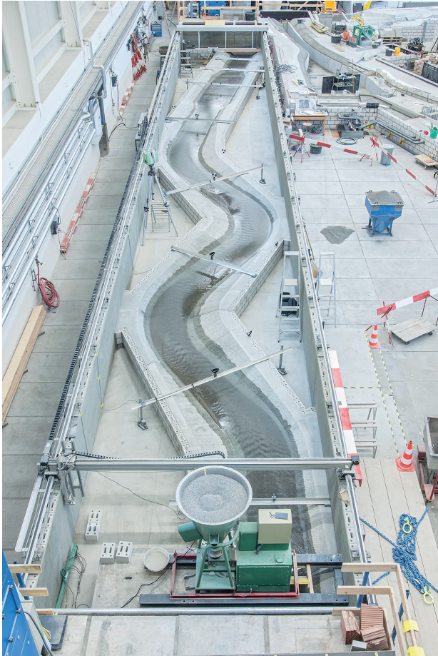
Scale model of the channel investigated (Picture: A. Schlumpf, VAW)
