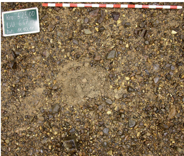
Figure 2: Underwater bed of River Rhine, photograph taken in a diver bell after volume sampling
