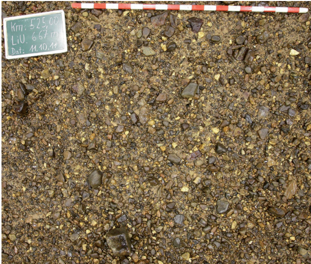
Figure 1: Underwater bed of River Rhine, photograph taken in a diver bell before volume sampling
