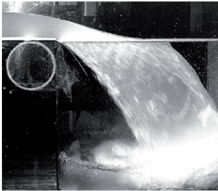
Typical Flow Structure
