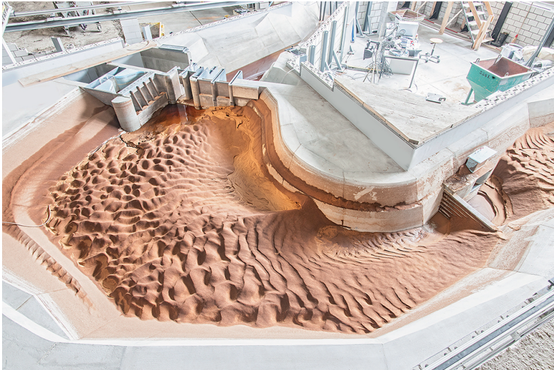
Investigation of a 20-year flood with suspended sediment load modelled with ground walnut shells.
