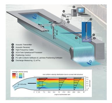
This PSEL research project rises the question of how to improve the efficiency of a desilting equipment. The research strategy is based on systematic experiments and on previous results collected by VAW during the past 3 decades. Experiments are conducted in situ at three different desilting chambers ( $L \times W \times H$ ; 28.1m, 36.0m, 60.0m x 4.5m, 9.0m, 7.5m x 6.61, 2.76, 6.89) at variable discharges. Different sediment flushing systems are considered.
