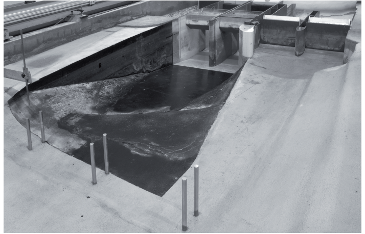
Fig.2: Hydraulic model of the power plant with its two turbines on the left and the flood weir on the right at a scale of 1:30
