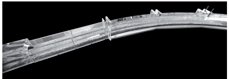
sediment transport in the bypass tunnel
