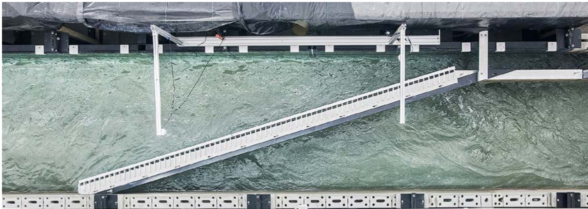
Fig. 1: Fish guidance structure in a laboratory flume at VAW
