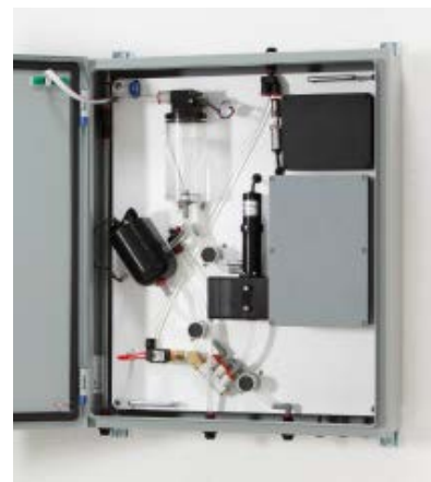
Fig. 2: In-situ laser diffractometer with automatic dilution chamber ( www.sequoiasci.com )
