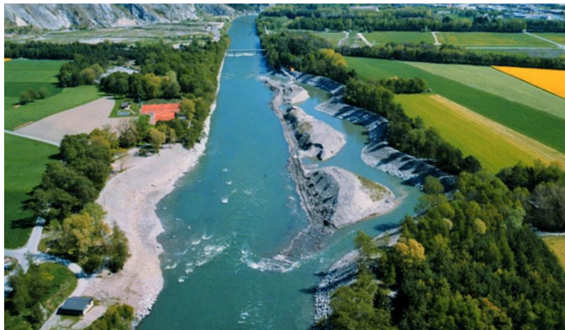
Fig. 1: A secondary channel as bank erosion inducement measure directly after the construction of the river widening Felsberg, Alpine Rhine River, GR ( www.alpenrheinschule.net )
