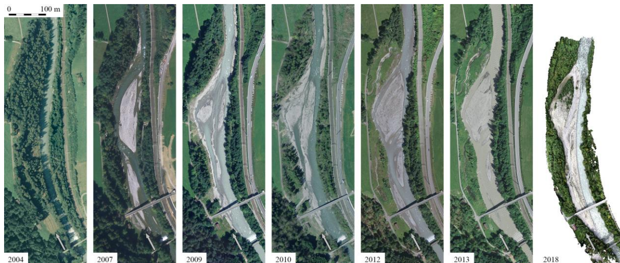
Fig. 1: Morphodynamic change in the dynamic river widening Heustrich at the Kander River. (2004-2013 © swisstopo, 2018 VAW)
