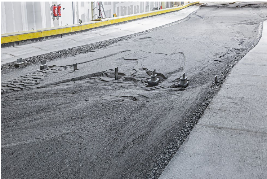
Fig. 1: Pillar scour as well as morphological scour in a hydraulic model test (Source: VAW)
