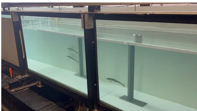
Fig 1: Photo of live-fish tests with Atlantic salmon in spring 2023 (left) and representative photo of an EGS with vertical-axis vortex generating elements (right)
