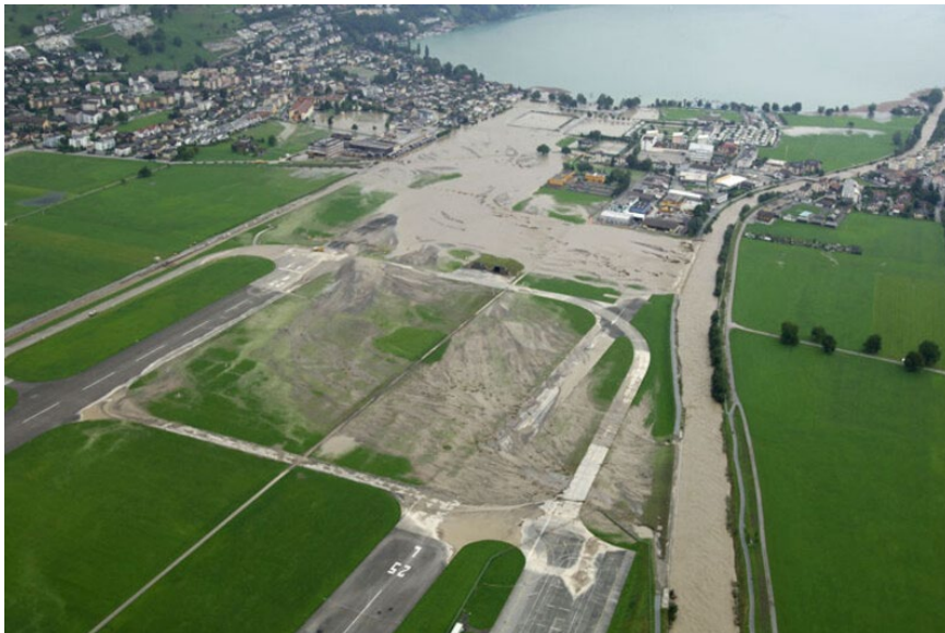
Fig. 1: Lateral diversion of discharge into flood corridor during major flood event 2005 at Ennetbürgen-Buochs (NW). (Source: planat.ch)
