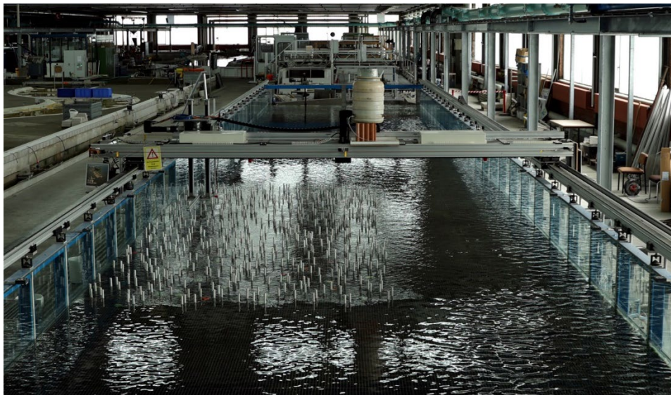
Fig. 1: Experimental flume setup with a Mid age floodplain forest (source: KIT)
