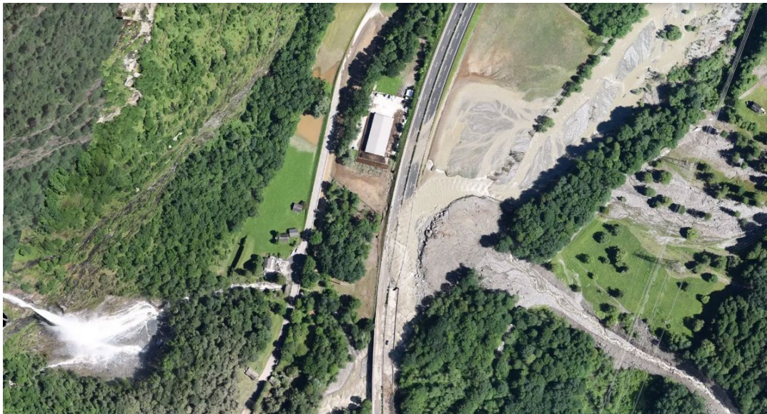
Fig. 1: Moesa river diversion due to debris-flow after heavy precipitation in the Valle Mesolcina in June 2024 (©swisstopo)
