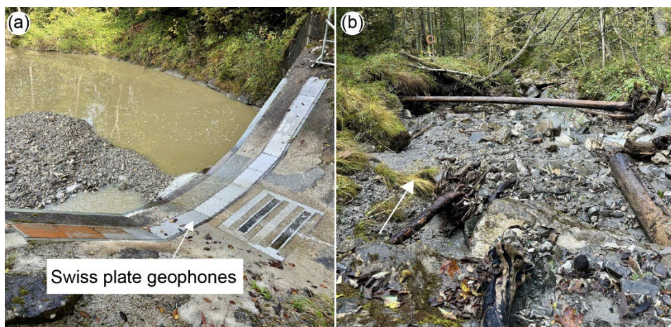
Fig. 1: (a) Installed SPGs and (b) impression of wood and bedload transport at the Erlenbach
