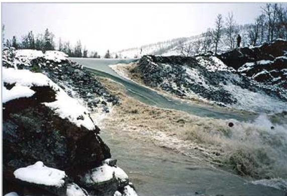
Abb. 1: Dam breach field test of a 6 m dam (left, source: IMPACT-project) and possible outflow hydrographs (right).
