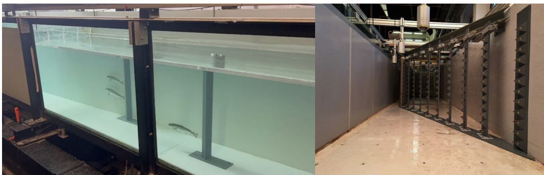
Fig 1: Photo of live-fish tests with Atlantic salmon in spring 2023 (a) and representative photo of an EGS configuration (delta wing element) in the etho-hydraulic flume (b)
