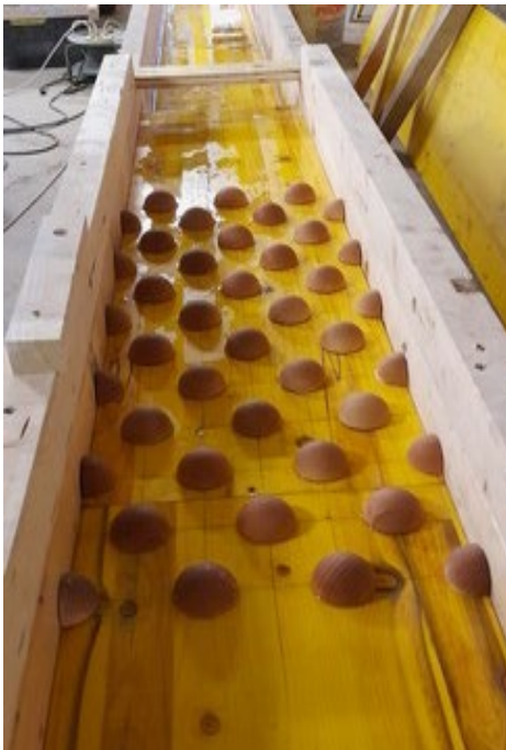
Fig. 1: Two views of the experimental flume at Laboratorium 3D in Biasca. In this case, the bed roughness is given by semi-spheres placed with a density of approximately 25%.
