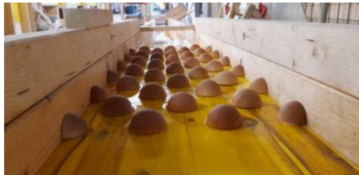
Fig. 1: Two views of the experimental flume at Laboratorium 3D in Biasca. In this case, the bed roughness is given by semi-spheres placed with a density of approximately 25%.
