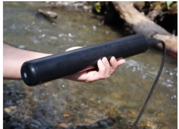
Fig. 2: Acoustic sensor for measurements of suspended sediment concentration (LISST-ABS) ( www.sequoiasci.com )
