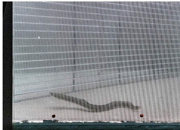
Fig. 1: Eel reacting to the electric field in the laboratory flume at VAW
