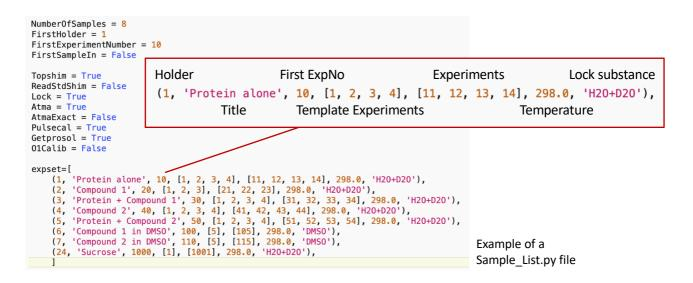
For starting the actual experiments, the user presses the "Run Experiment Series" button. At this point the Sample\_List.py file will be written again and the RunSeries.py script will be called.
