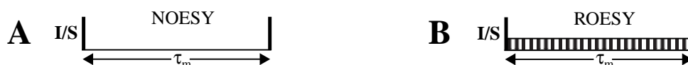
Fig. 15. Schemes for a homonuclear NOESY (A) and ROESY (B) transfer segment. For short mixing times \tau_m ( \tau_m typically smaller 40 ms) the transfer from S magnetization to I magnetization, \Delta I , is usually proportional to the S spin magnetization at the start of the mixing time, S^0 (Eq. (2.12)): \Delta I = \tau_m \sigma_N S^0 for NOESY and \Delta I = \tau_m \sigma_R S^0 for ROESY.
