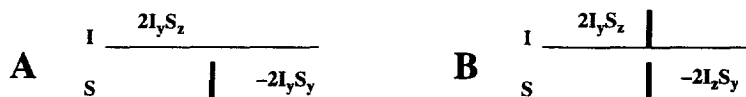
Fig. 16. Schemes for heteronuclear polarization transfer starting from heteronuclear anti-phase magnetization. Narrow vertical bars stand for 90^\circ RF pulses. The cartesian product operators indicated in the figure describe a typical coherence transfer step to heteronuclear multiple quantum (A) and to heteronuclear single quantum coherence (B). Transformation properties in the shift operator basis are given in Table 9.
