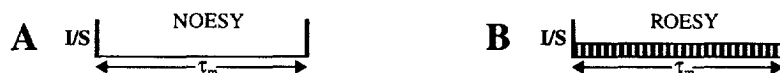
Fig. 15. Schemes for a homonuclear NOESY (A) and ROESY (B) transfer segment. For short mixing times \tau_m ( \tau_m typically smaller than 40 ms) the transfer from S magnetization to I magnetization, \Delta I , is usually proportional to the S spin magnetization at the start of the mixing time, S^0 (Eq. (12)): \Delta I = \tau_m \sigma_N S^0 for NOESY and \Delta I = \tau_m \sigma_R S^0 for ROESY.
