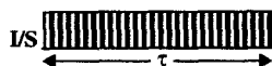
Fig. 14. Scheme for a homonuclear TOCSY transfer segment. During \tau the spins I and S are spin-locked with a strong RF field which makes magnetization transfer from the I to the S spin possible, and vice versa, according to Eq. (9).
