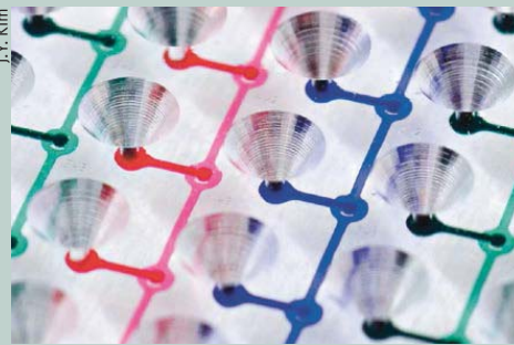
The micro-tissues in these chambers are provided with metabolites and messenger materials through the coloured channels.
