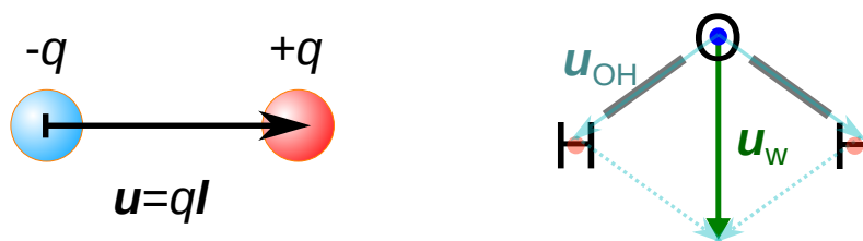
Figure 9.2: The dipole. Left: the dipole moment u is defined pointing from -q to +q . Right: the dipole moment u_w of water, is the sum of the bond dipole moments u_{OH} .
