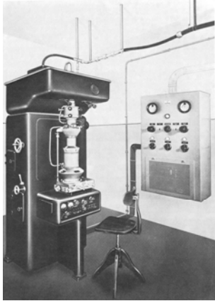
1939: first TEM serially produced by Siemens resolution ca. 7 nm
