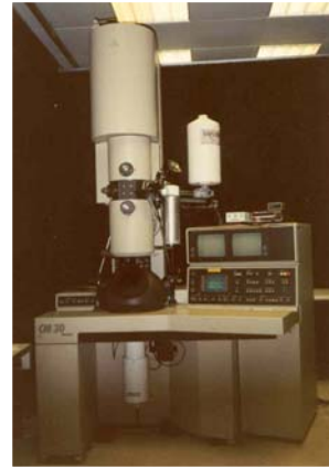
~1990 Philips CM30, V = 300 kV resolution ca. 0.2 nm
