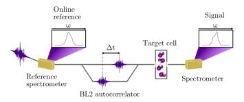
FIG. 1. Sketch of the experimental setup. The incoming FEL spectrum is parasitically measured via the VLS online spectrometer [36]. The main beam then passes the FLASH BL2 autocorrelator [35] to split the beam into pump and probe pulses with a variable time delay  $\Delta t$  between them. These pulses are focused into the interaction volume (target cell, filled with gas-phase di-iodomethane), and the probe transmission spectra are detected as a function of the pump-probe time delay.
