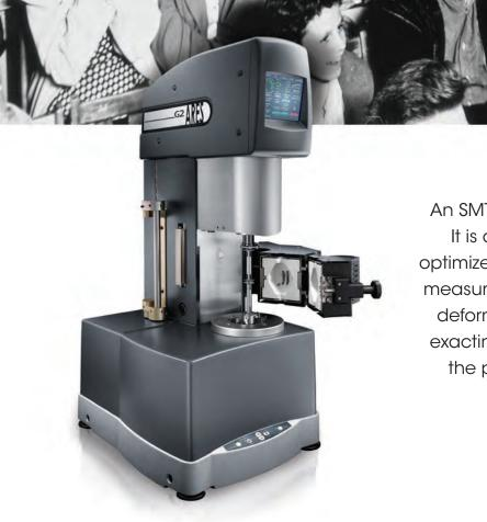
An SMT rheometer is more than two drives. It is a separate motor and transducer optimized for every aspect of the rheological measurement. A motor designed for perfect deformations. A transducer optimized for exacting stress measurements. The result is the purest rheological measurements.
