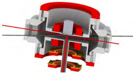
FIG. 1: Experimental schematic, showing laser cooling beams impingent on a cloud of atoms trapped 800\mu\text{m} away from a thin vacuum window and a microscope objective.
