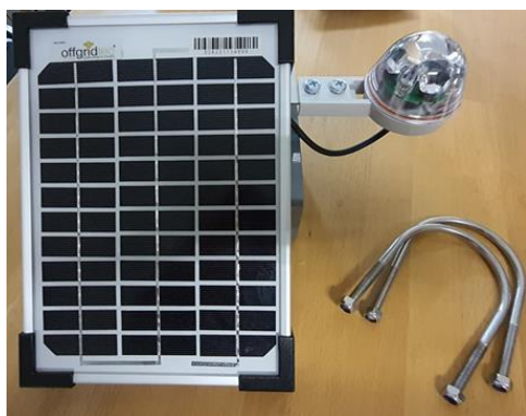
Fig 1: The NIVUS rain sensor system with infrared sensor, PV element and LoRaWAN sender.
