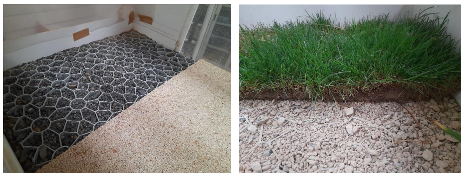
Fig 2: Two permeable pavement solutions installed in the laboratory testbed, with a honeycomb grid and resin-gravel pavement (left-hand panel) and with meadow (right-hand panel).
