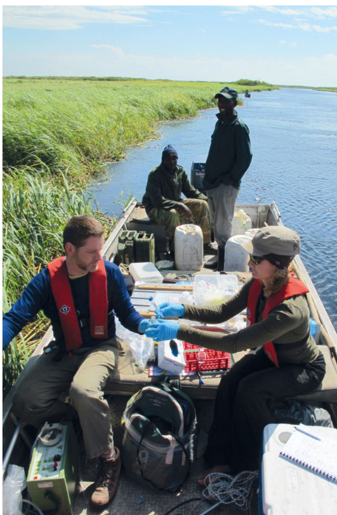
ADAPT: The African Dams Project: Adapt planning and operation of large dams to social needs and environmental constraints – an integrated water resource management study in the Zambezi basin. Filtering water samples for nutrient analysis at headwaters of Kafue River, Zambia.
