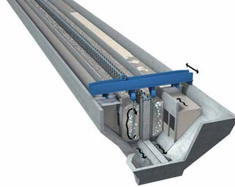
Grease and oil removal at the surface through aeration and fine sand trap at the bottom.
