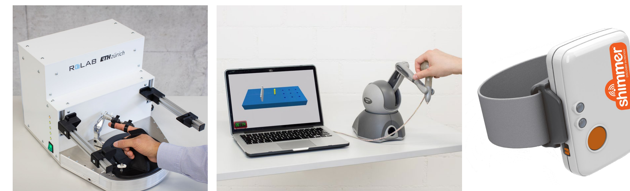
Figure 2: Three different technologies are used in the FHT longitudinal study to accurately and sensitively track the recovery after stroke. That includes the ETH MIKE, the Virtual Peg Insertion Test (VPIT) and wearable sensors (Shimmer).
