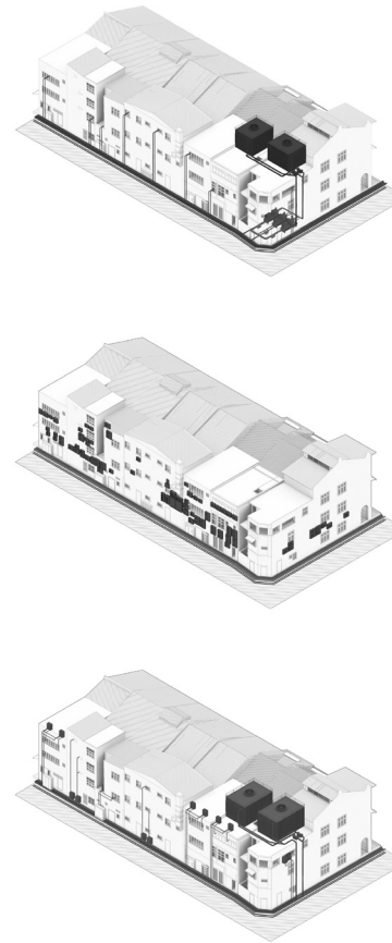
Cooling systems: centralised, decentralised, heat bus (top-bottom)
