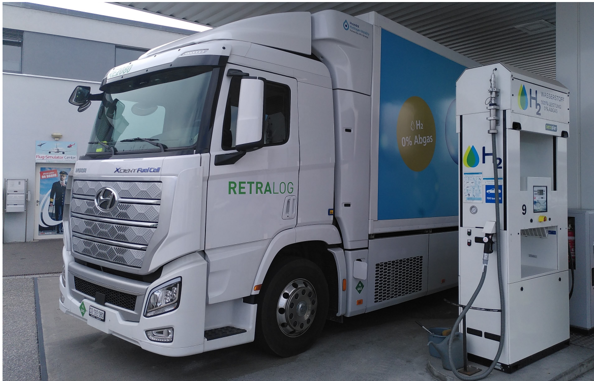
Figure B.1: Fuel cell electric rigid truck at a hydrogen fueling station (Picture: Andreas Eckmann)
