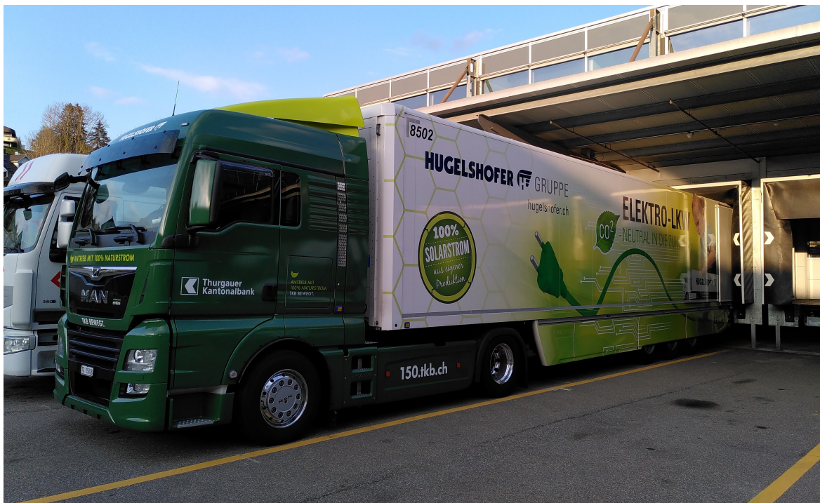
Figure B.2: Battery electric articulated tractor-trailer truck at a logistics center (Picture: Andreas Eckmann).
