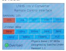
For such installations this Remote Control Interface (SP 983a) is a helpful device. It allows controlling the gain and the low-pass filter cut-off frequency remotely and it also displays the status of the Overload LED.
