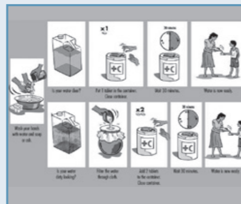
4.8 Treating water with chlorine To shows students how to apply chlorination tablets or solution to treat water.
