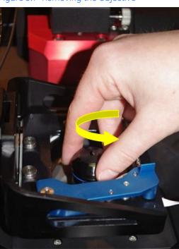
Figure 3.7 Removing the Objective
