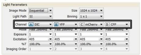
5. Select the correct camera **Mode** for each active channel. Each mode setting consists of two values: channel mode and readout speed.
