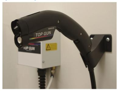
All functionality is built into the gun, including a flow control value for adjusting the airflow, a balance adjustment for calibration, and a two-level LED. The air gun has a filter at its exit to ensure that out-flowing air is clean.
