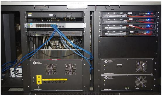
Figure 3.2 Electronics Rack - Block Drawing - Shown with Four Camera Workstations
