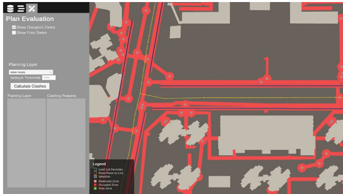
Fig.3 Review of minimum required clearance from regulatory areas and existing underground infrastructure
