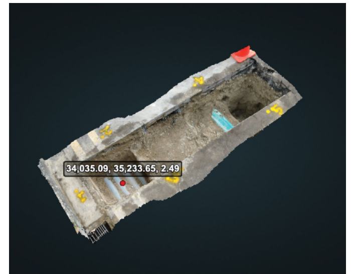
Point cloud of captured trial trench with georeferenced coordinates
