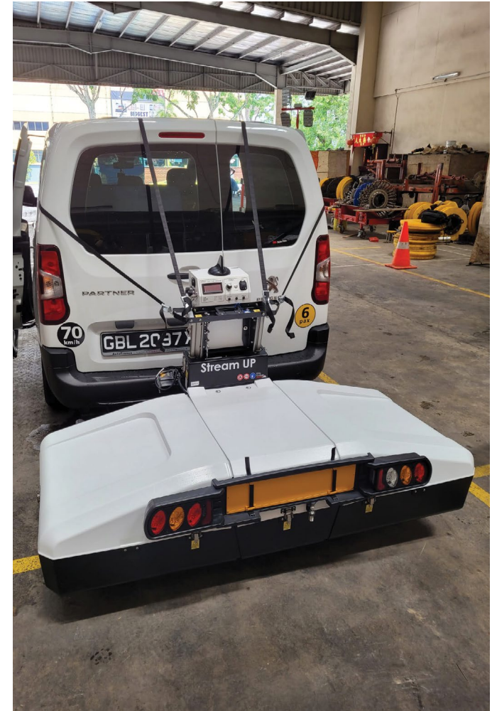
IDS GeoRadar Stream Up ready for testing in Singapore
