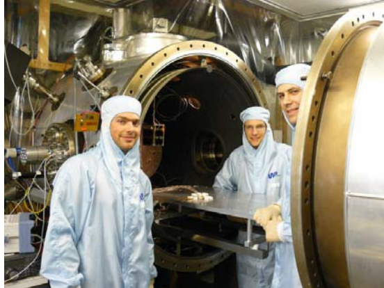
Figure 18: Test preparation for the Thermal Vacuum Cycling test at Uni-Berne.
