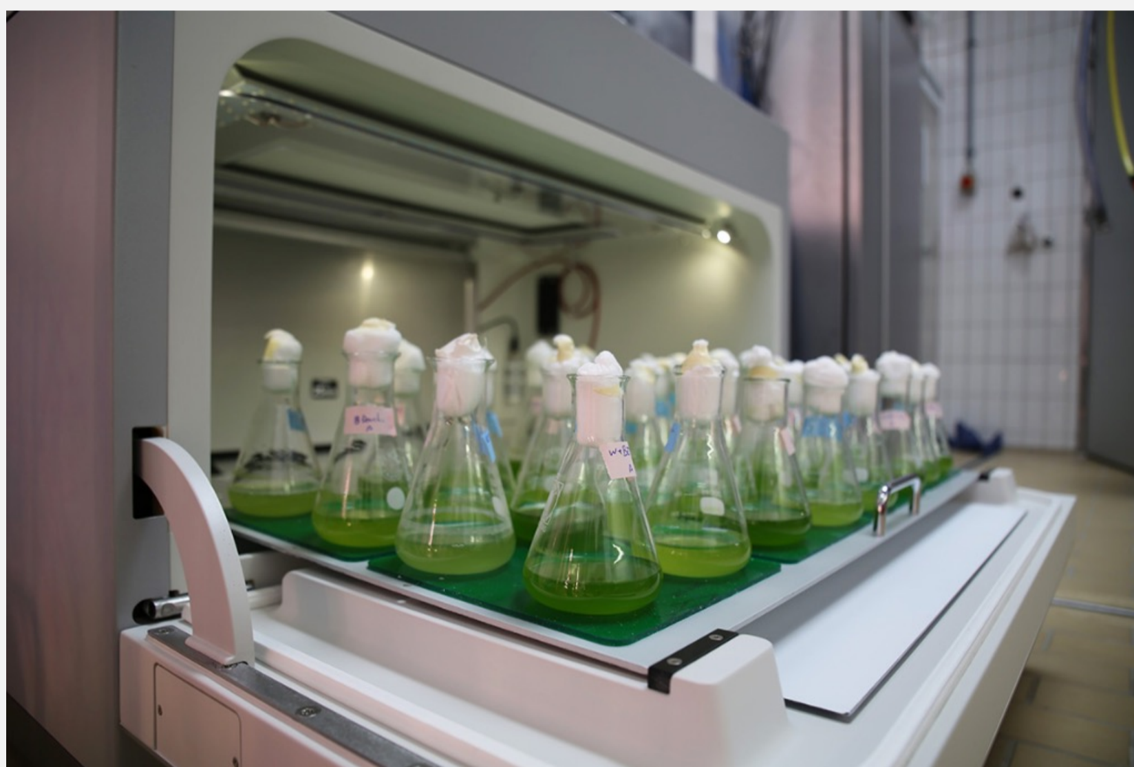
Figure 1. Microalgae cultures in Erlenmeyer flasks growing in the CO 2 incubator, light at 115 μmol/m 2 .s in a 16h:8h day/night photoperiod cycle at optimal temperature, shaken at 110 rpm.
